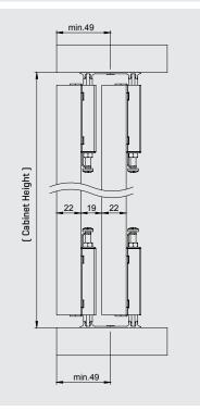
NOTE DIMENSIONS, SHOWN IN BRACKETS ARE VALID FOR "18 mm" AND "22 mm" DOOR THICKNESSES.
